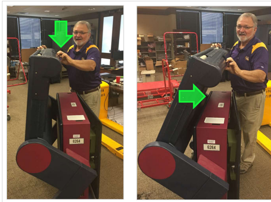
Figure 20: Pull Maroon Latch on Tub and Tilt to the Upright Voting Position
